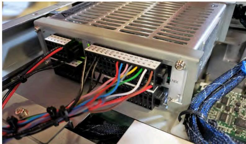
**f** Make your own cabling for the three wires going from the safety enclosure to the XGPIO interface module.
