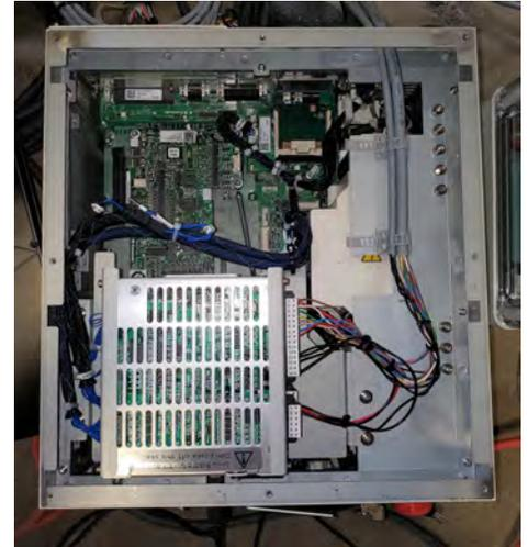
**e** Connect the safety controller output wires to the destinations on the Cubic-S terminals and the safety enclosure.
